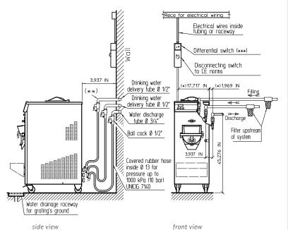
(\*) Even if the machine models vary, the water and electricity connection positions are always the same, i.e. on the LEFT side of the machine.
