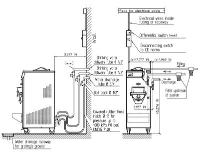
(\*) Even if the machine models vary, the water and electricity connection positions are always the same, i.e. on the LEFT side of the machine.
