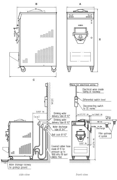
(\*) Even if the machine models vary, the water and electricity connection positions are always the same, i.e. on the LEFT side of the machine. (\*\*) Cocks are in vertical only for illustration purposes. (\*\*\*) 30 mA (ABB serie C).
