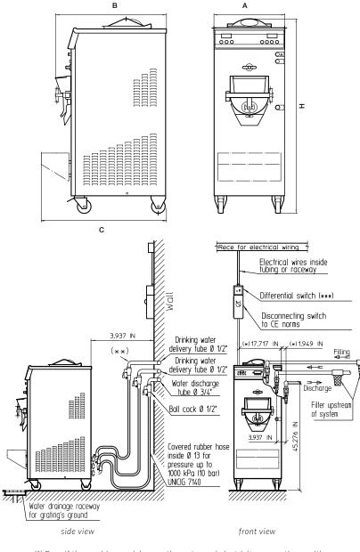
(\*) Even if the machine models vary, the water and electricity connection positions are always the same, i.e. on the LEFT side of the machine. (\*\*) The cock is higher for illustration requirements. In really it must be placed side by side with the other. (\*\*\*) 300 mA (ABB serie K)
