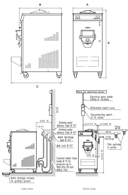
(\*) Even if the machine models vary, the water and electricity connection positions are always the same, i.e. on the LEFT side of the machine. (\*\*) Cocks are in vertical only for illustration purposes. (\*\*\*) 30 mA (ABB serie C).
